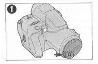
\*Press part A to remove the lens cap.
