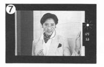
\*When correct focus has been achieved (autofocus indicator has lit up), press the shutter release button fully. As soon as the shutter is released, the film will automatically advance to the next frame.
