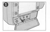
\*Open the mode cover and press the DRIVE button until "D.EXP." is displayed on the LCD panel.
