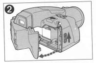
\*Open the back cover by sliding the back cover release.
