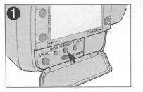
\*Open the mode cover and press the SUBJECT button until ? is displayed on the LCD panel.
