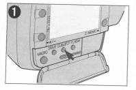
\*Open the mode cover and press the SUBJECT button until (1990) is displayed on the LCD panel.
