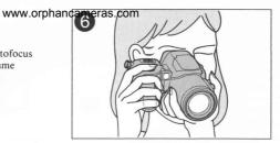
\*Press the shutter release button halfway to focus.
