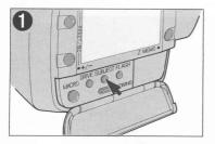
\*Open the mode cover and press the SUBJECT button until 💟 is displayed on the LCD panel.
