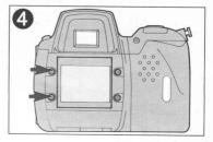
\*Press the mode button and the +/- button simultaneously to check the remaining battery power.
